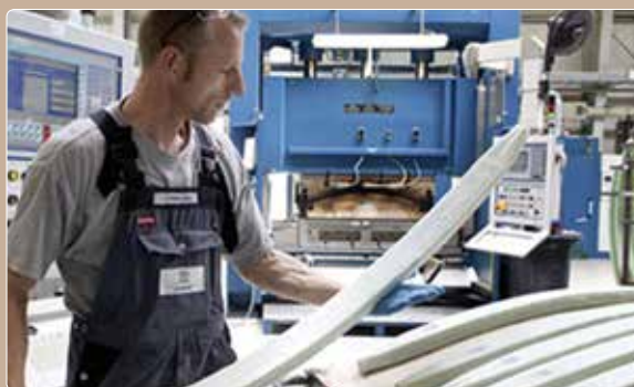
IFC Composites (Haldensleben, Germany) has been mass-producing glass-reinforced epoxy-based leaf springs since 2005. The company uses a prepreg manufacturing system, and has supplied more than 1.3 million composite leaf springs for light duty trucks, including Daimler's Mercedes-Benz Sprinter cargo van (top photo). ■
