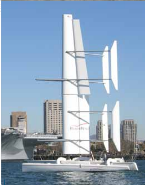
The HWT X-2, docked (top) and undergoing sea trials in California (bottom). Note the "balance beaks" protruding in front of the wing sail, which hold the electronic equipment that controls the two wing tails, to the rear of the wing. ■
