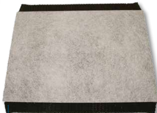
Commercial load floors and sunshades are now in production, made via a Composite Spray Molding process, using Bayer MaterialScience's (Pittsburgh, Pa.) Baypreg polyurethane resin system. Pictured here is a test panel, showing the assembled glass mat/paper honeycomb package before spraying. ■
