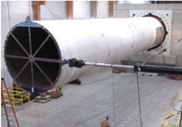
DeepCWind partners have already tested an Ershigs-built 1:2-scale bolted composite tower (one tower section is shown during testing). ■
