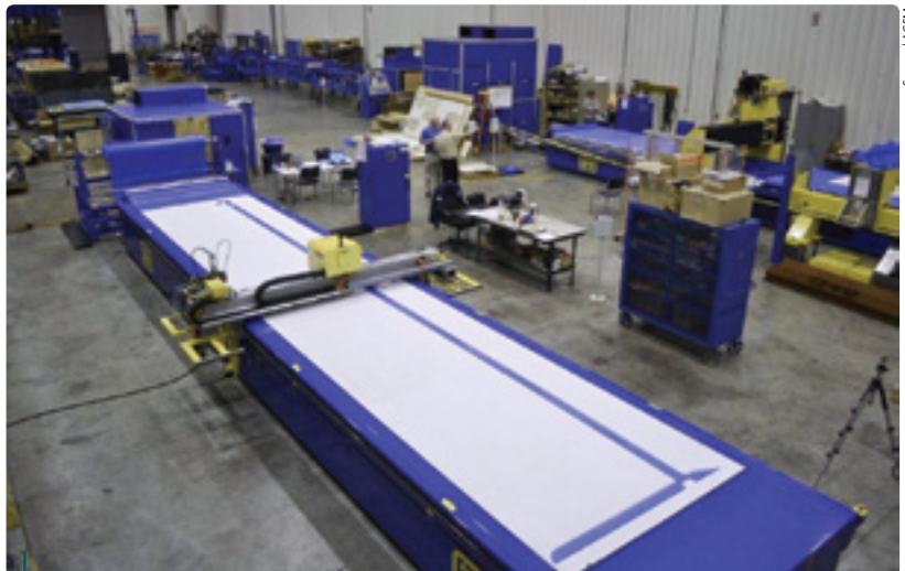
American GFM (AGFM, Chesapeake, Va.) and parent company GFM GmbH (Steyr, Austria), offer several types of composites-related machine tools, including this model US-15 flatbed ultrasonic ply cutter, with a 32-ft/9.75m cutting length. ■
