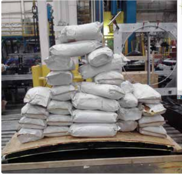
C-shaped double-arched composite roof bows, from CPI Binani (Winona, Minn.) are replacing aluminum I-beams in tow-behind RVs produced by Keystone RV Co. (Goshen, Ind.). Produced via D-LFT transfer molding, using chopped glass wetout with a recycled polypropylene copolymer blend, the bows feature insert-molded pine wood blocks on both ends, which simplify hand sizing and installation, using screws or nails. Photo at left shows bows during static load testing. ■
