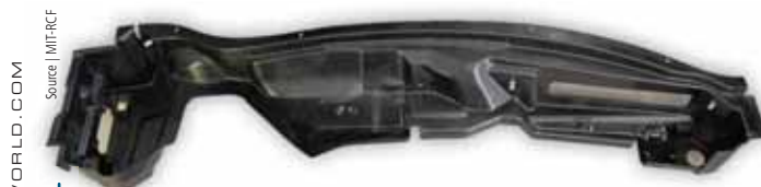
Fig. 4: Recycler MIT-RCF (Lake City, S.C.) converts chopped RCF into 3-DEP preforms, continuous nonwoven roll goods and pellets for LFT. Applications successfully demonstrated include automotive parts like the door bolster support for the Ford Escape and the 2014 C7 Corvette ’s upper plenum (pictured here). ■
