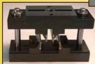
Three and Four Point Short Beam Fixture ASTM D 790, D 6272, D 7264
