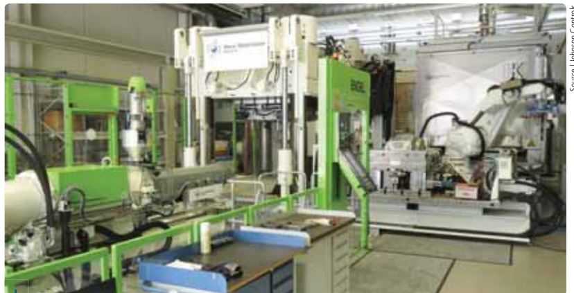
CAMISMA's automated production line includes (from background right to left foreground) an oven for preheating preforms, robotic transfer to SpriForm tool, conveyor transport of SpriForm tool to thermoforming press (white), and injection molding unit (green and gray, near left). ■
