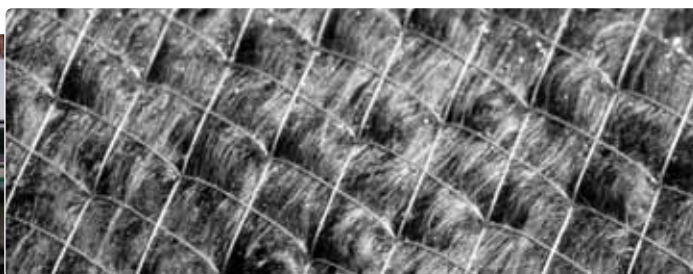
SGL Automotive Carbon Fibers (Wackersdorf, Germany) processes CF scrap from weaving and preform kitting operations for reuse in the BMW i -series CFRP Life Module. Reclaimed fiber is incorporated into stitched nonwoven materials (above), which are then molded into the i3 's rear seat structure and roof sections for both the BMW i3 (left) and i8 . ■
