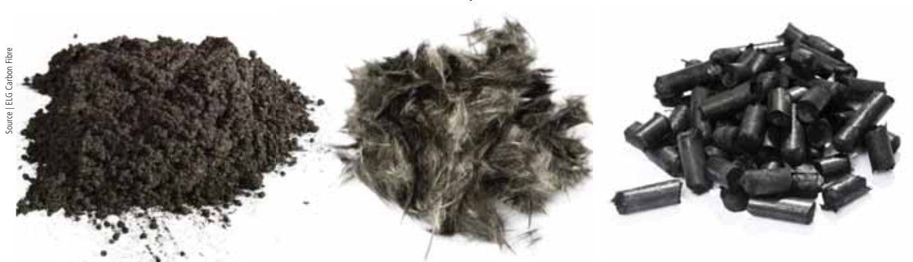
Fig. 2: Recycler ELG Carbon Fibre (Coseley, U.K.) produces milled fiber (left, with average length of 100µ); chopped fiber (center, with random lengths (6 to 60 mm)); and lightly compacted thermoplastic pellets (right) made with milled or chopped fiber and matrix-compatible binders. ■
